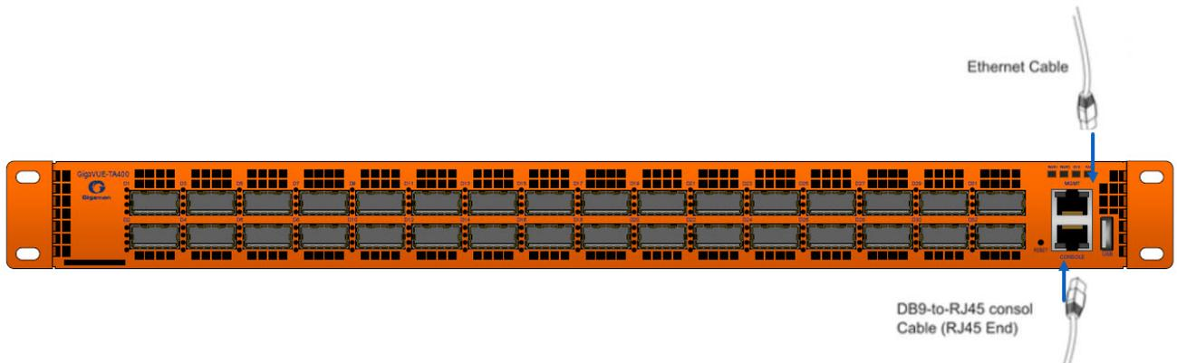
**Figure 15** Connecting the Console and Management Ports
