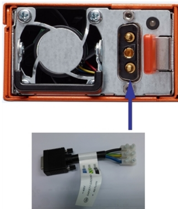
Figure 4 Connecting DC Power Supply Module
