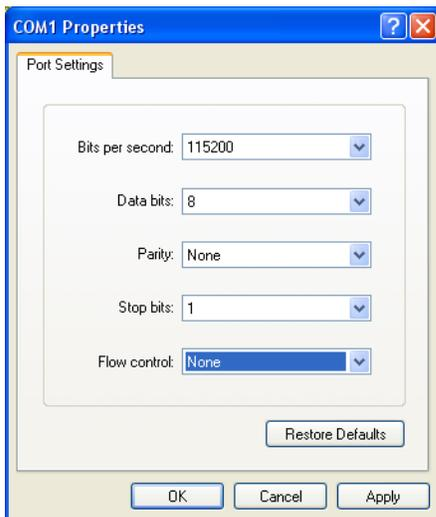
Figure 21: Setting COM Port Properties for the Console Connection
