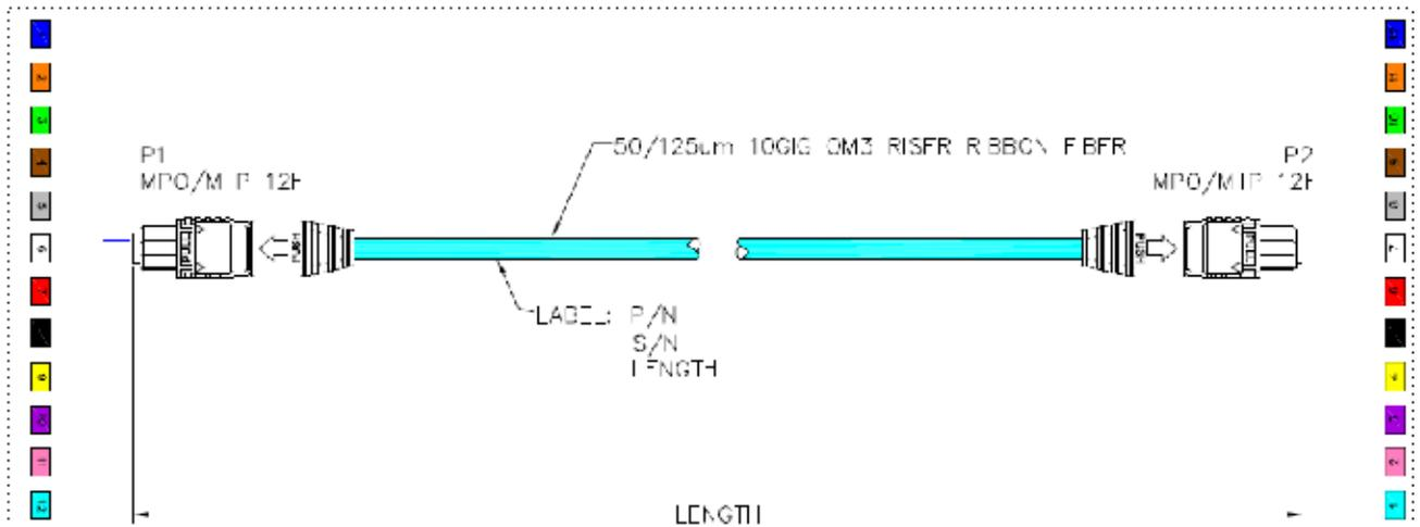
Figure 26: MPO/MTP 12 Position Fiber Cable
