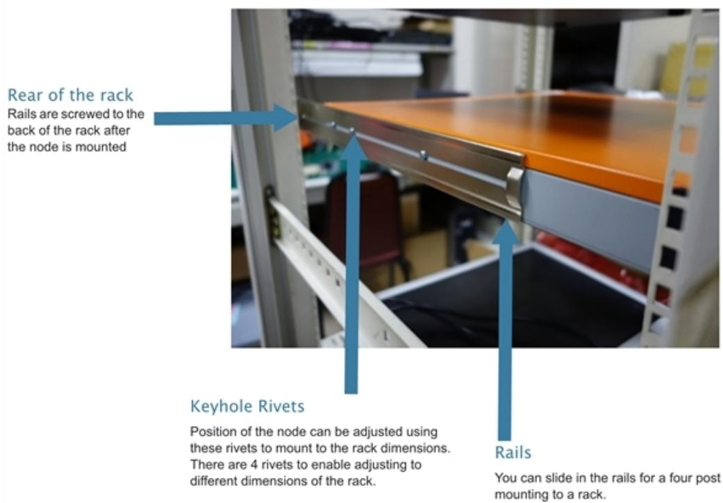
Figure 10: GigaVUE Traffic Aggregator with Rail Mounting for Four-Post Racks
