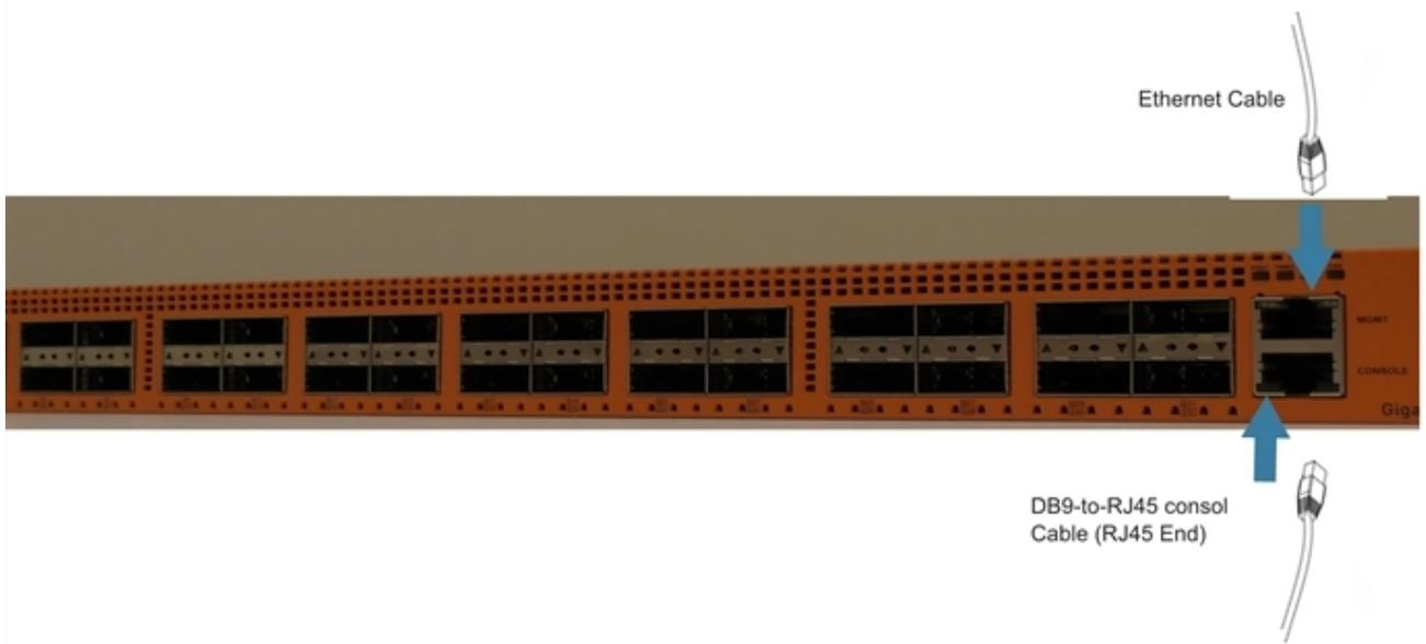
Figure 20: Connecting the Console and Management Ports
