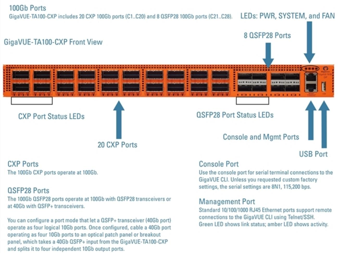
Figure 4: The GigaVUE-TA100-CXP Chassis Front View
