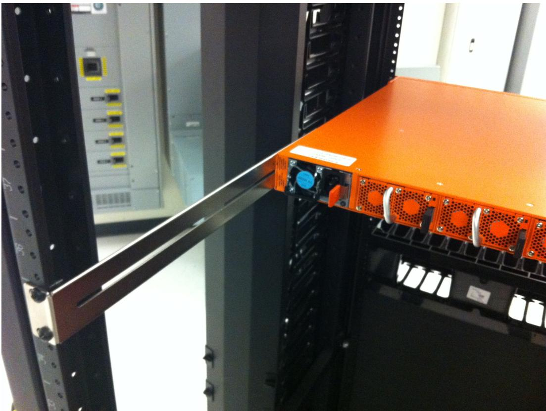
*Figure 12: Rear View of the Mounted Node and Rails on the Four-Post Rack*
