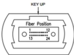
Figure 28: MPO/MTP 24 Position Fiber Cable
