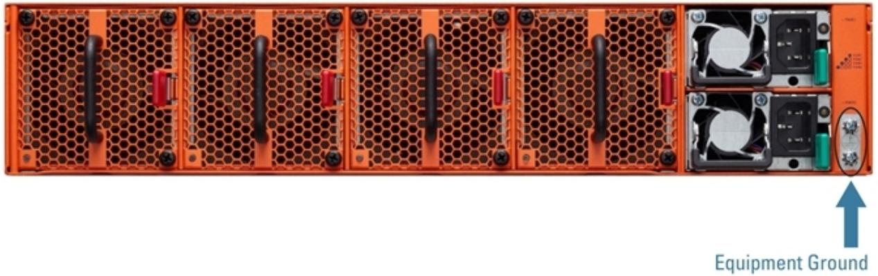
Figure 14: Ground Screws (GigaVUE-TA200 Shown)
