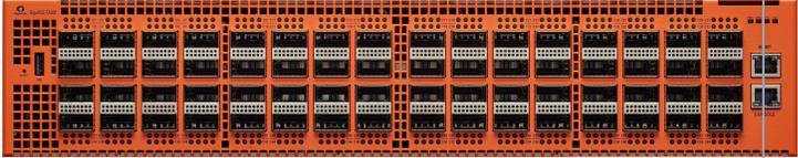
A 2RU network node with 64 100Gb/40Gb ports, shown as a long orange PCB with multiple port modules.                              |
