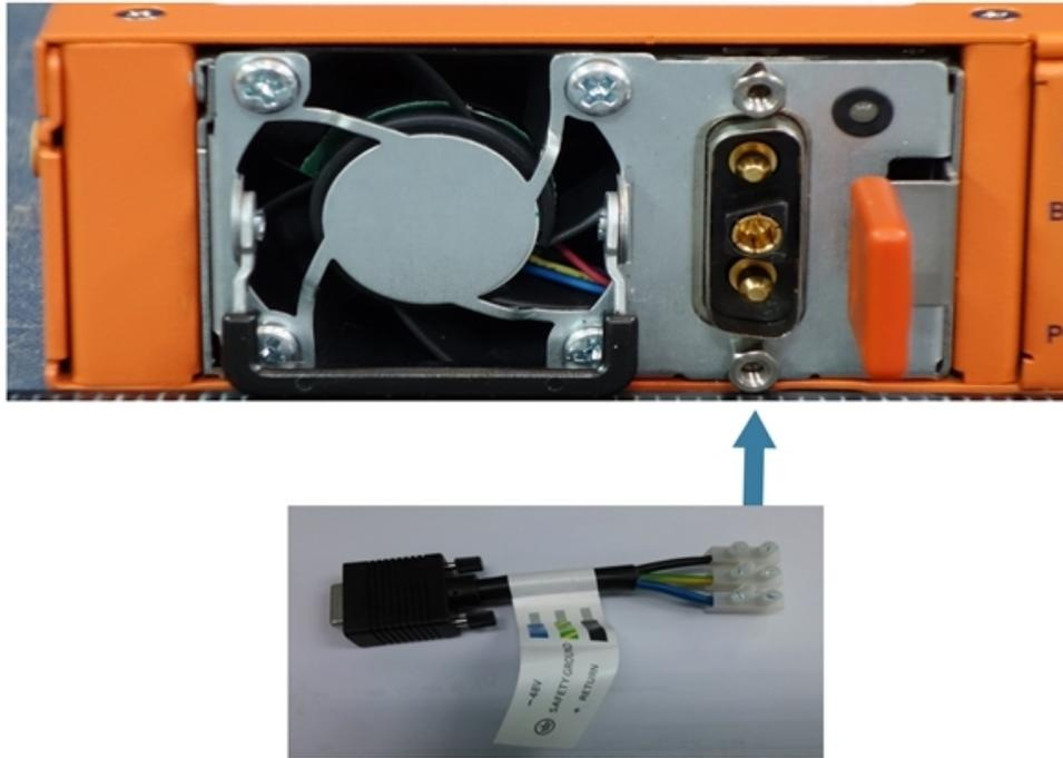
Figure 18: Connecting -48V DC Power Cable Adapter
