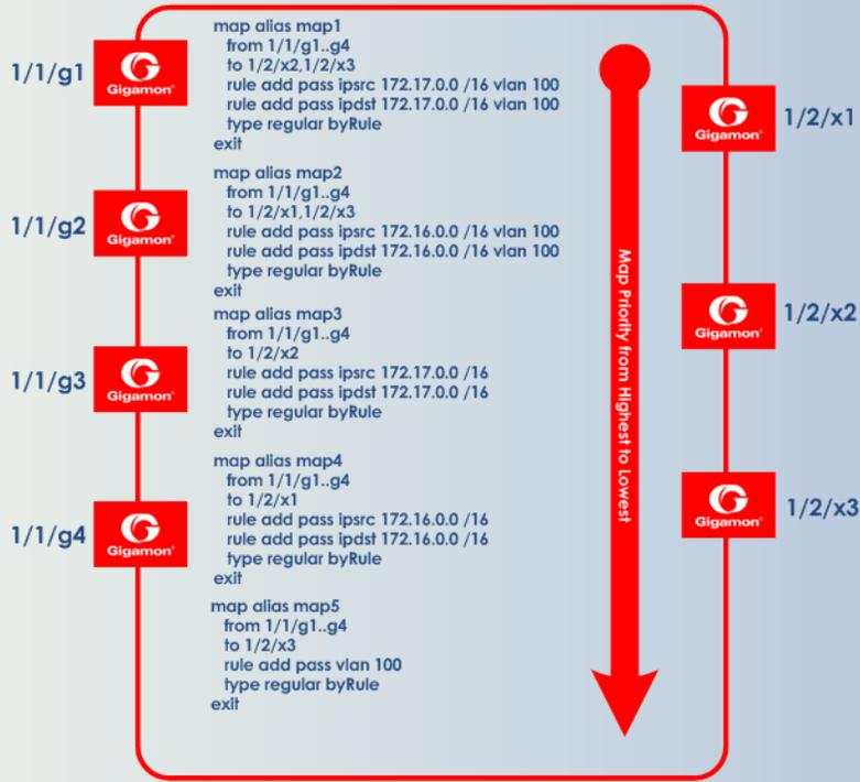
Figure 4: Sending Subnets and VLANs to Different Ports
