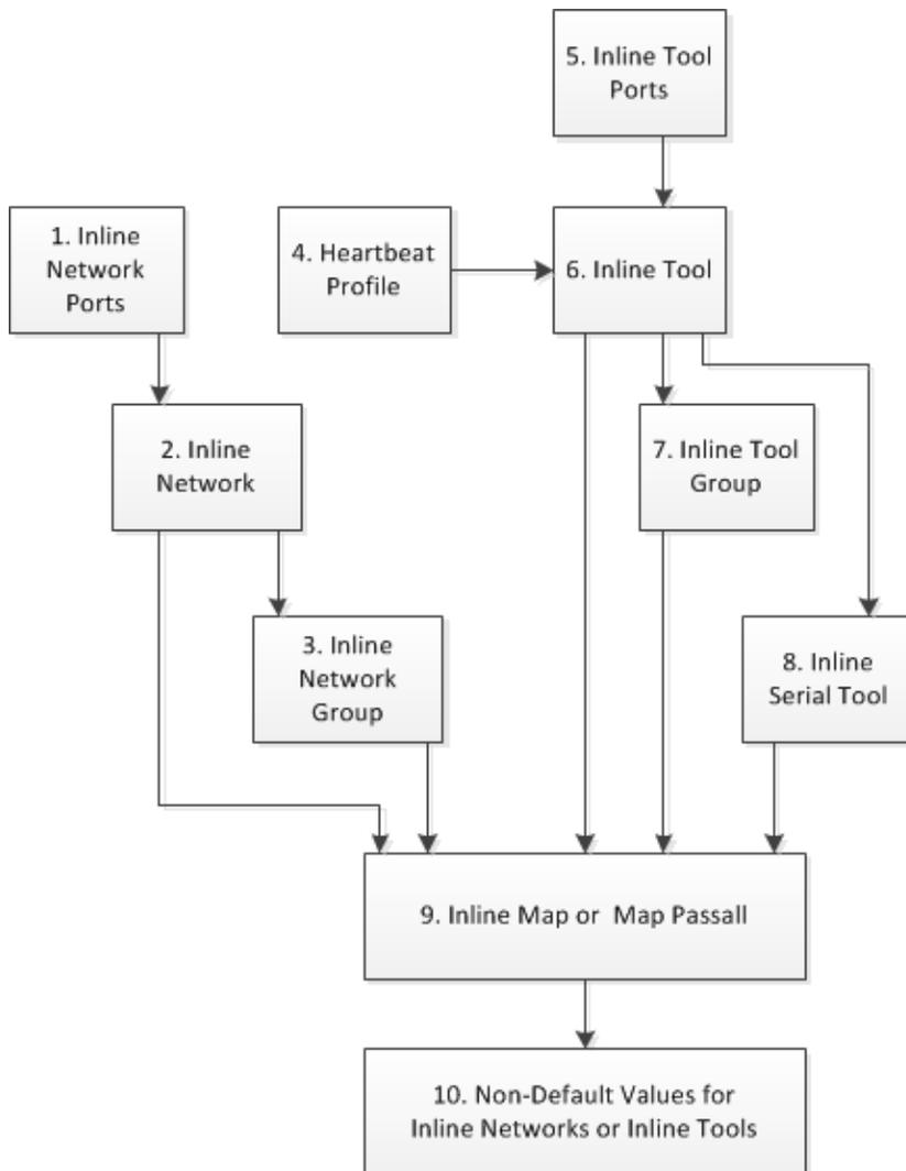
Figure 10: Configuration Steps for Inline Bypass Solutions
