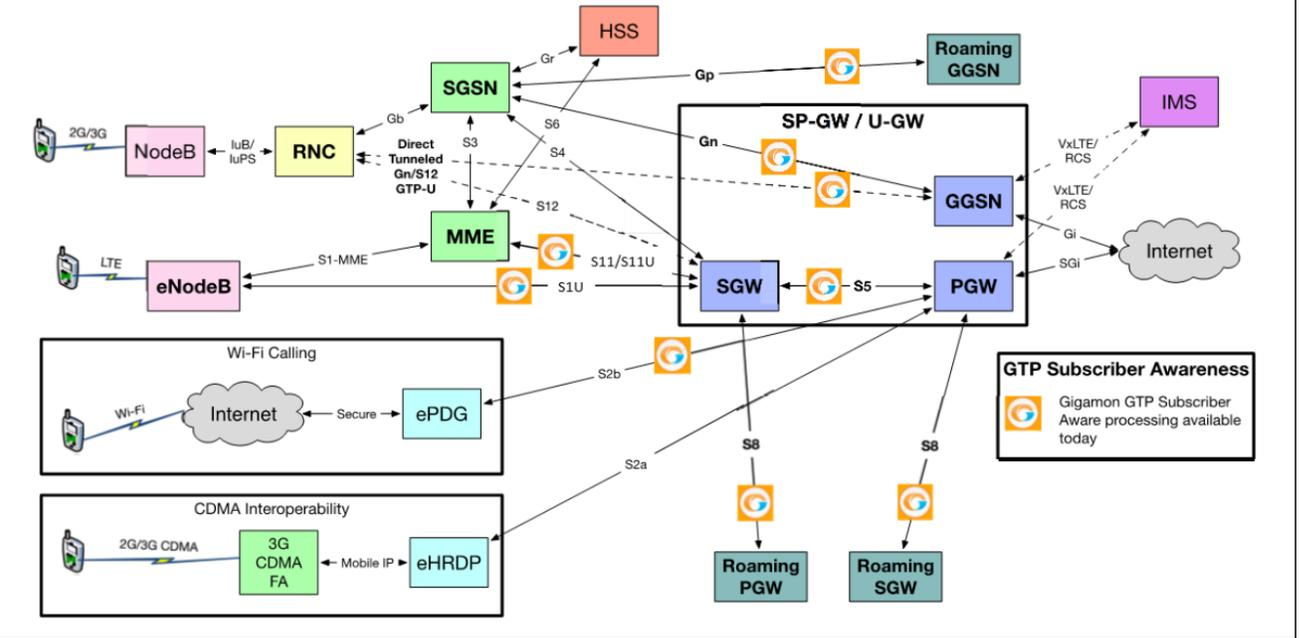
In Example 1, filter rules are configured to identify and forward all the traffic related to subscribers identified by an IMSI prefix. All traffic specific to the filtered IMSI's 2222222222223\*, including GTP-c and GTP-u, is forwarded to a monitoring tool. A shared collector is configured to which traffic not matching the filters is sent.
