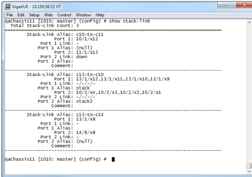
Figure 26: Output of show stack-link for Sample Cluster
