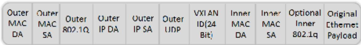
**NOTE:** This can be applied to any protocol that is supported through header stripping. GTP, VXLAN, ISL, MPLS, MPLS+VLAN, VLAN, VN-Tag, and fabric-path are all supported, as is Gigamon tunnel decapsulation.
