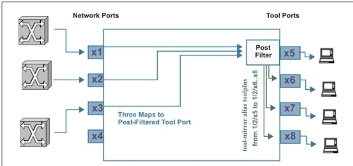
Figure 9: Adding tool-mirrors to Multiple Tool Ports
