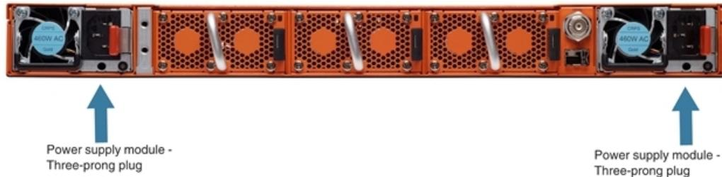
Figure 2: Connecting AC Power
