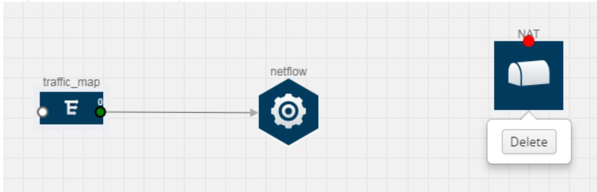
9. Create a link from the v5 NetFlow application to NAT. The link must be configured with the destination IP address of the NetFlow collector and the GigaVUE V Series node interface. For steps to configure the link, refer to [Link NetFlow Application to NAT](#).
