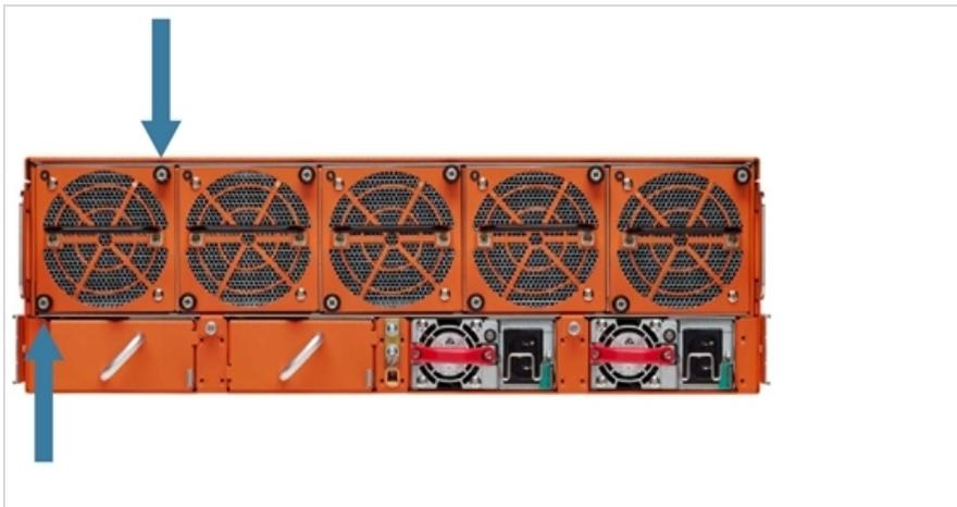
Figure 7: Fan Module Screw Location on GigaVUE-HC3 Rear
