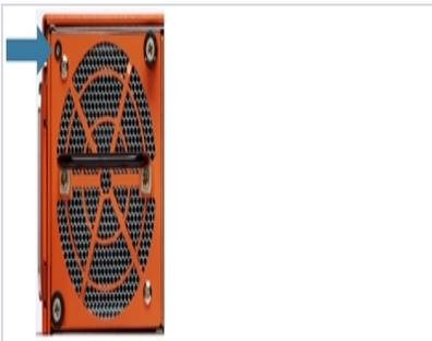
Figure 6: Individual Fan LED Location on GigaVUE-HC3 Rear
