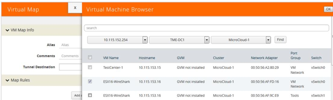
Figure 14: Selecting Virtual Machine Network Adapter
