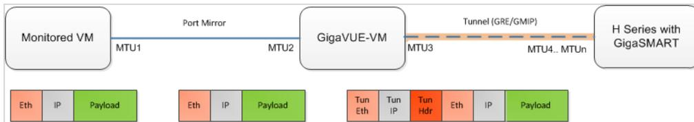
Figure 1: Fragmentation on GigaVUE-FM Tunnels in VMware Environments
