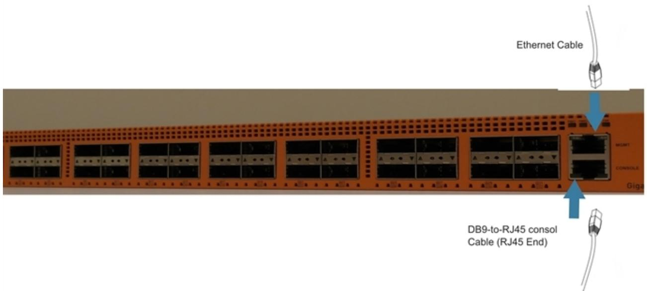
**Figure 15** Connecting the Console and Management Ports
