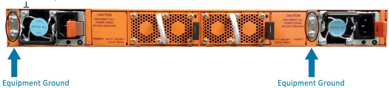
**Figure 8** Ground Screws (GigaVUE TA Series-TA10 Shown)
