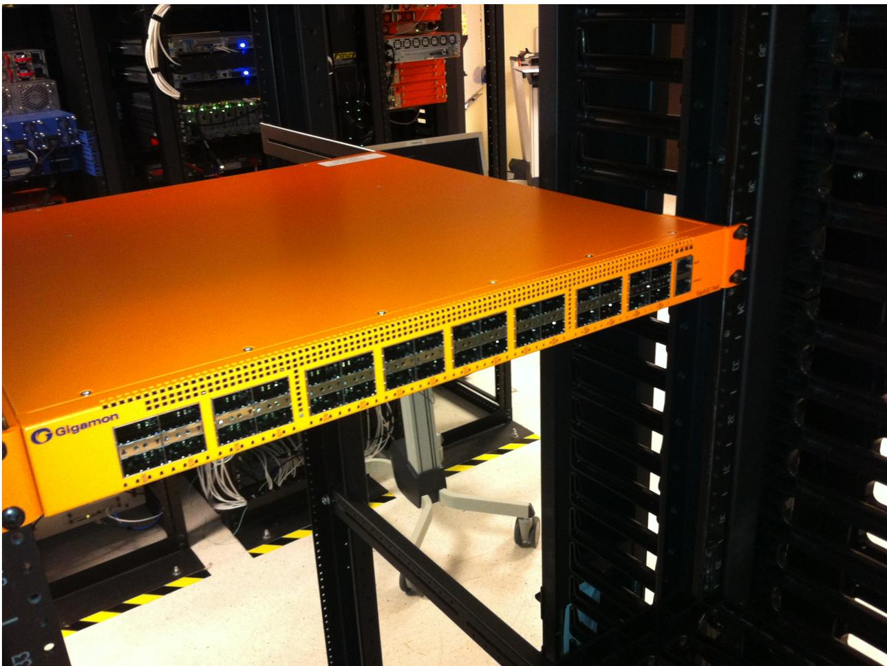
**Figure 6** Front View of the Mounted Node to the Four-Post Rack
