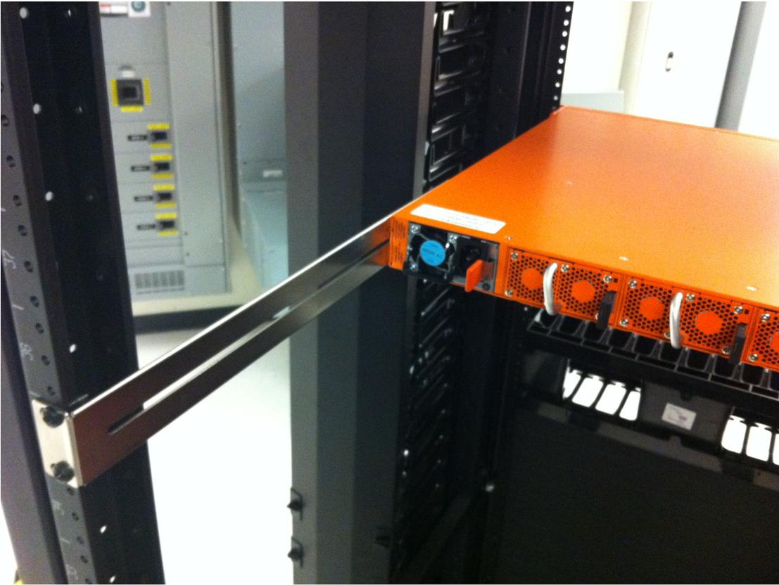
**Figure 7** Rear View of the Mounted Node and Rails on the Four-Post Rack
