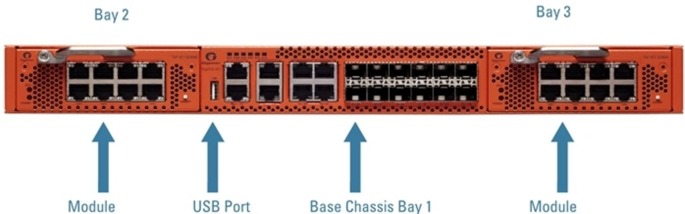
**Figure 1** Front View of the GigaVUE-HC1 Chassis
