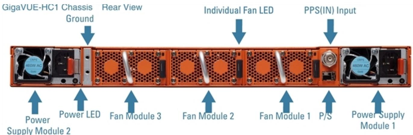
**Figure 2** Rear View of the GigaVUE-HCI Chassis
