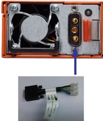
**Figure 4** Connecting DC Power Supply Module
