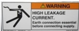
The GigaVUE-HC1 chassis is drilled for ground screws near the left corner at the rear of the chassis. Connect grounding wire with spade lugs to the ground screws on the chassis and earth ground using the following procedure.
