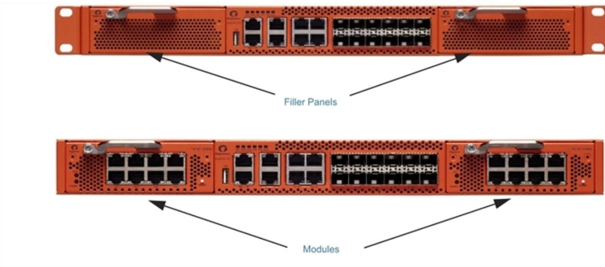
**Figure 4** *Installing Modules*
