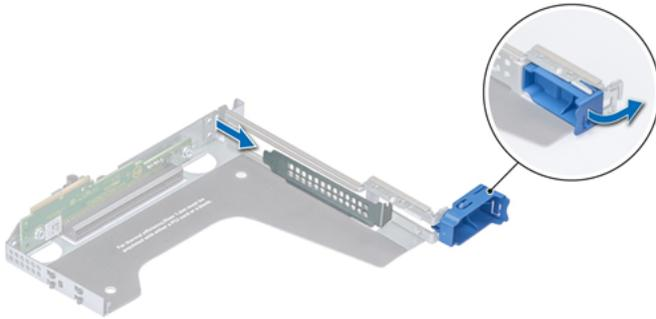
3. Hold the card by its edges, and align the card edge connector with the expansion card connector on the riser.
