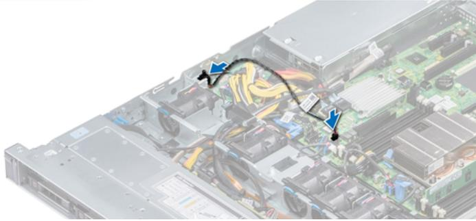
2. Slide the intrusion switch until it is firmly seated in the intrusion switch slot.
