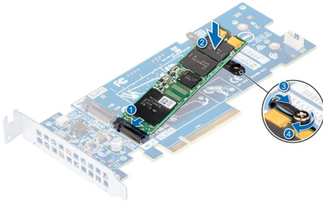
After installing the M.2 SSD module you could do the following:
