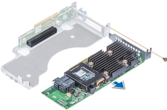
After removing the PERC card from the Internal PERC Riser you could do the following:
