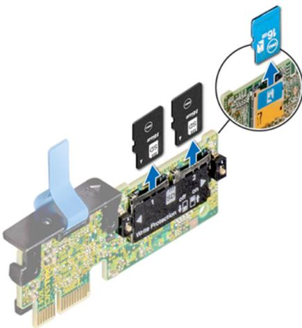
**NOTE:** Temporarily label each MicroSD card with its corresponding slot number after removal.
