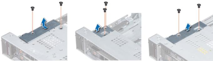
3. Using a Phillips #1 screwdriver, remove the screws that connect the control panel to the system.
