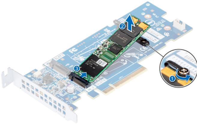
After removing the M.2 SSD module you could do the following:
