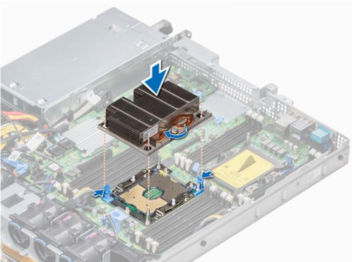
After installing the Processor Heat Sink Module follow the procedure listed in [After working inside your system](#).
