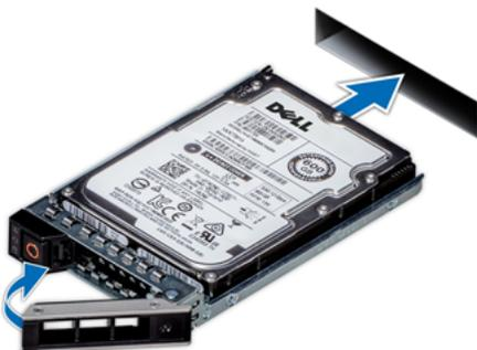
After installing the Hard Drive if applicable, install the front bezel.
