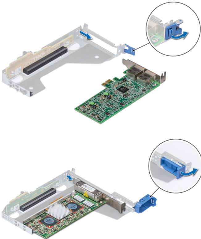
3. Install a filler bracket if you are not replacing the expansion card.
