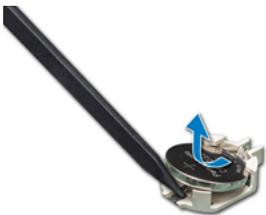
3. To install a new system battery, hold the battery with the positive side facing up and slide it under the securing tabs.
