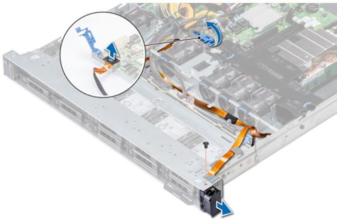
4. Holding the control panel by its sides, remove the control panel away from the system.
