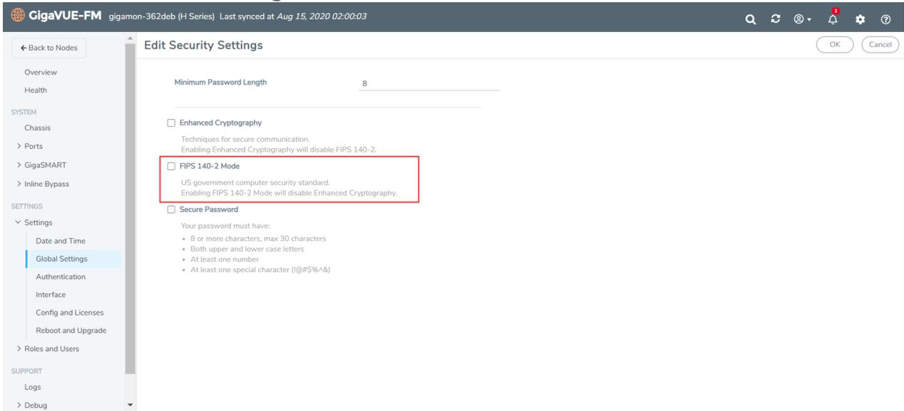
Once FIPS is enabled, the device will reload and the device configuration will be reset. All traffic, keys and certification configurations will be cleared.
