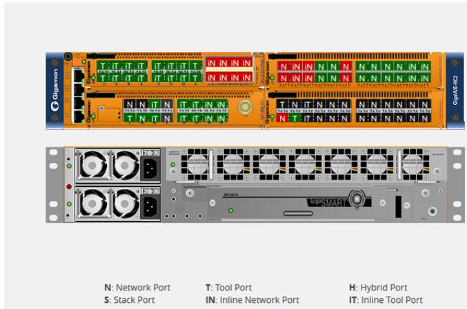
**Figure 20** Chassis View + Type View
