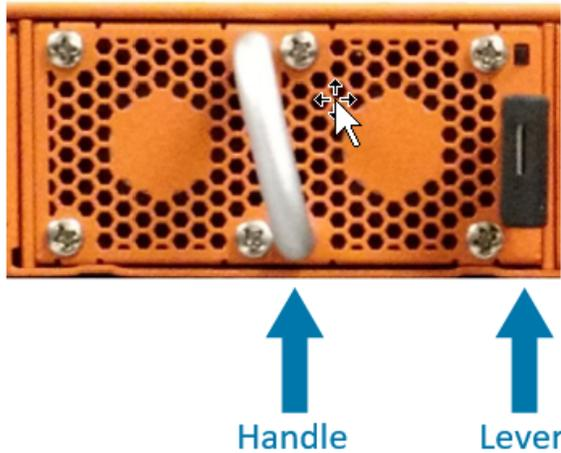
**Figure 20** Replacing a Fan (GigaVUE TA Series-TA10 Shown)
