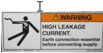
The GigaVUE TA Series chassis is drilled for ground screws at the rear of the chassis. Connect grounding wire with spade lugs to the ground screws on the chassis and earth ground using the following procedure.
