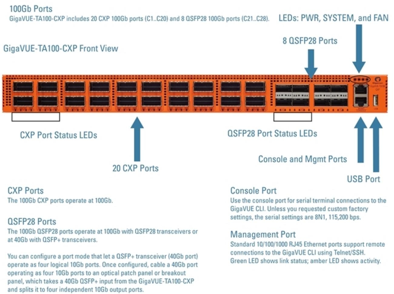
**Figure 5** The GigaVUE TA Series-TA100-CXP Chassis Front View
