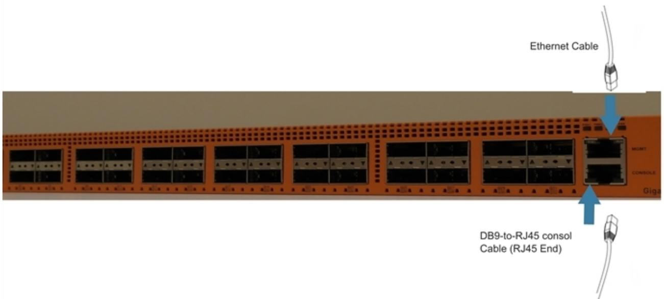
**Figure 21** Connecting the Console and Management Ports
