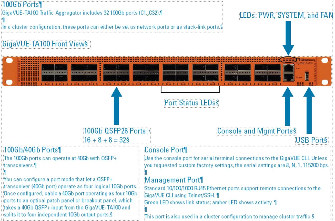
**Figure 3** The GigaVUE TA Series-TA100 Chassis Front View
