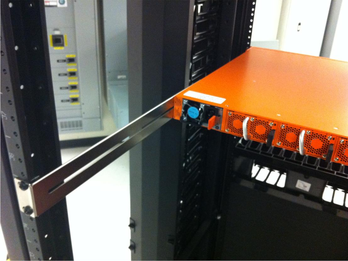
**Figure 13** *Rear View of the Mounted Node and Rails on the Four-Post Rack*
