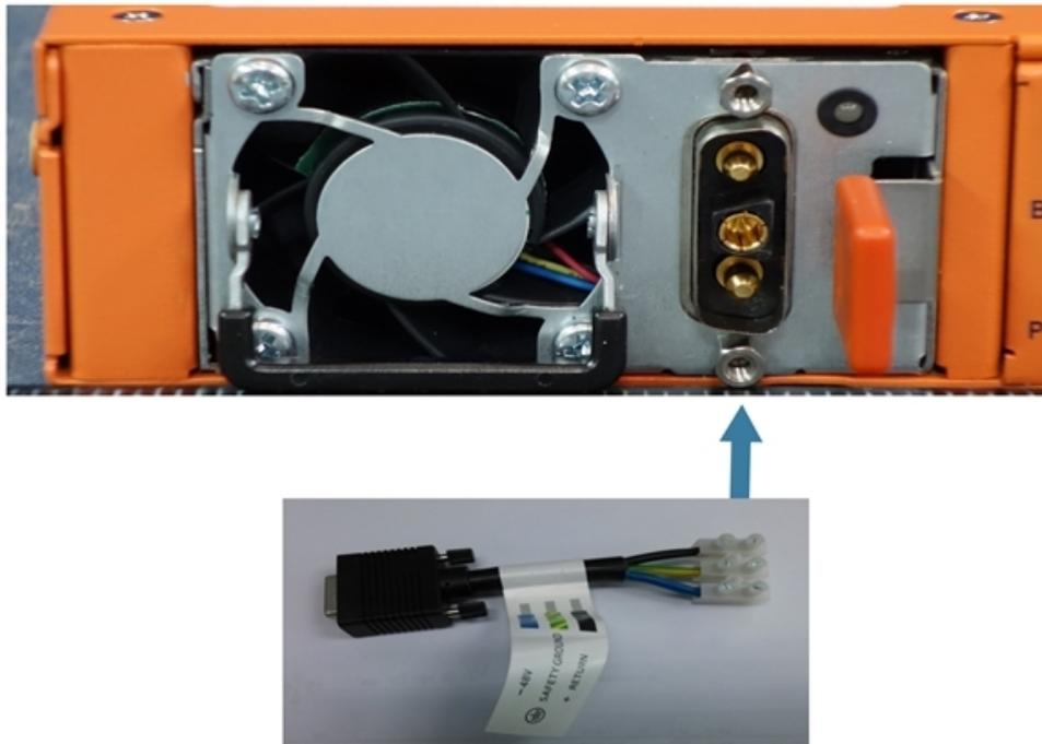
**Figure 19** Connecting -48V DC Power Cable Adapter
