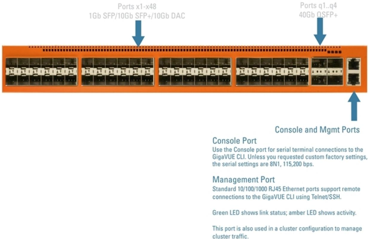
**Figure 1** The GigaVUE TA Series-TA10 Chassis
