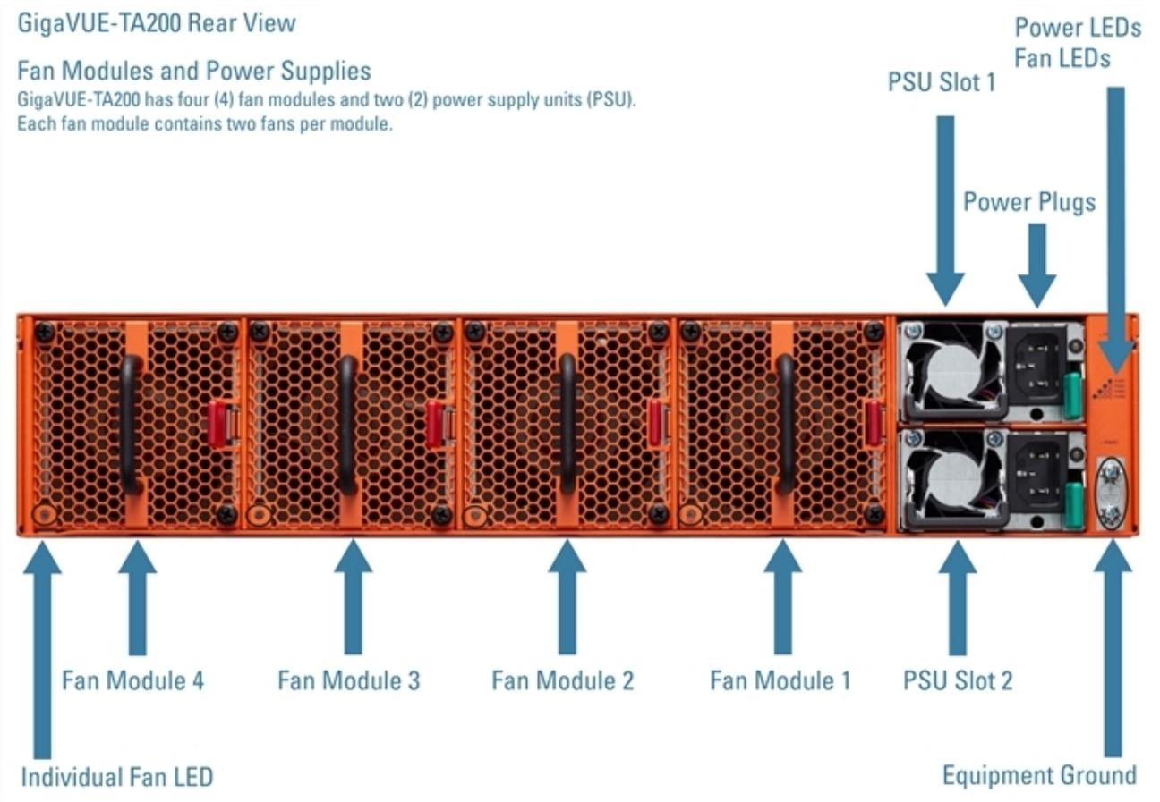
**Figure 8** The GigaVUE TA Series-TA200 Chassis Rear View
