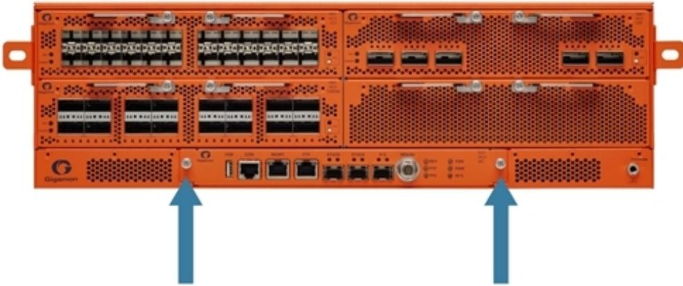
**Figure 15** Extension Board Screw Location on GigaVUE-HC3 Front
