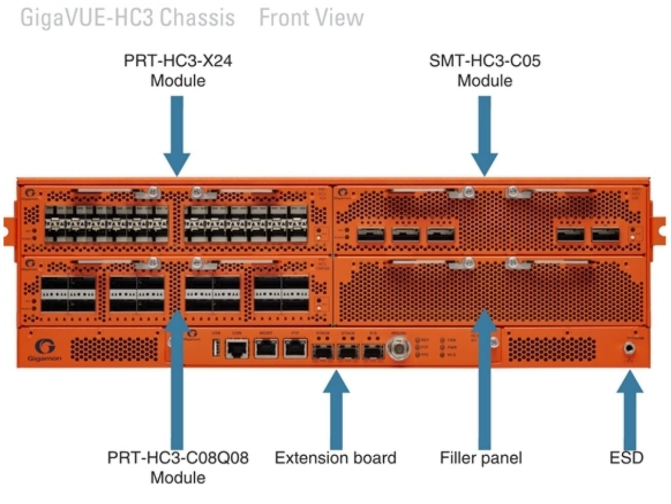
**Figure 2** Front View of the GigaVUE-HC3 Chassis
