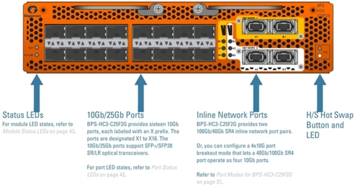
Figure 9 BPS-HC3-C25F2G Module
