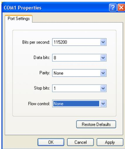
**Figure 23** Setting COM Port Properties for the Console Connection
