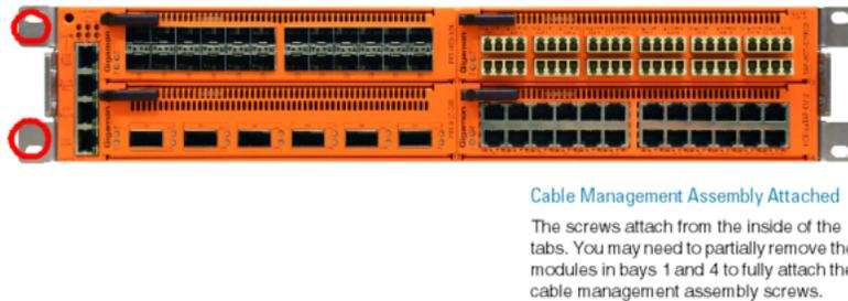
**Figure 8** Cable Management Assembly Attached to Node
