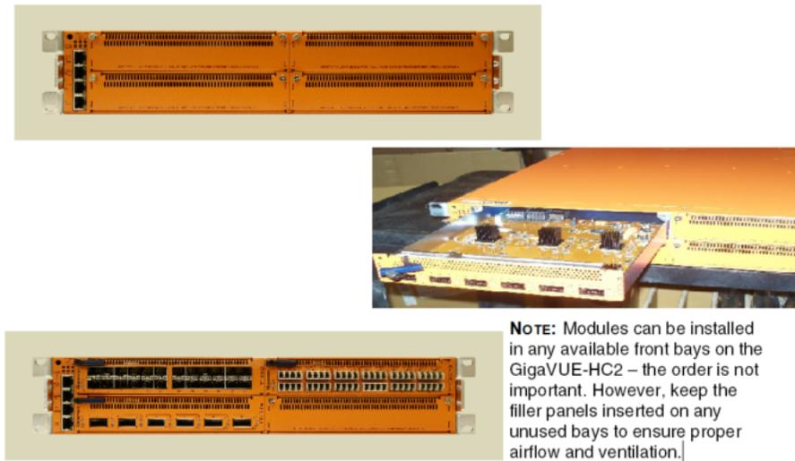
**Figure 11** *Installing Modules*
