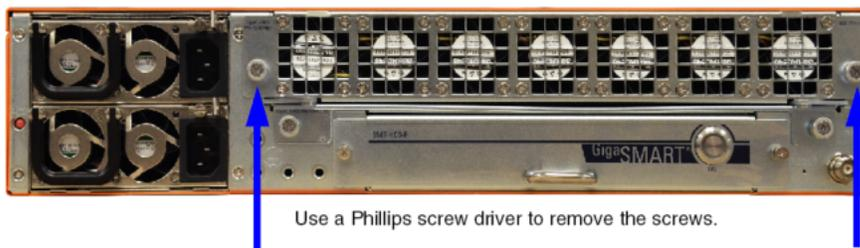
4. Remove two lower screws as shown in the following figure.
