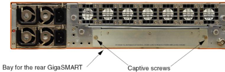
The rear GigaSMART module is installed as follows:
