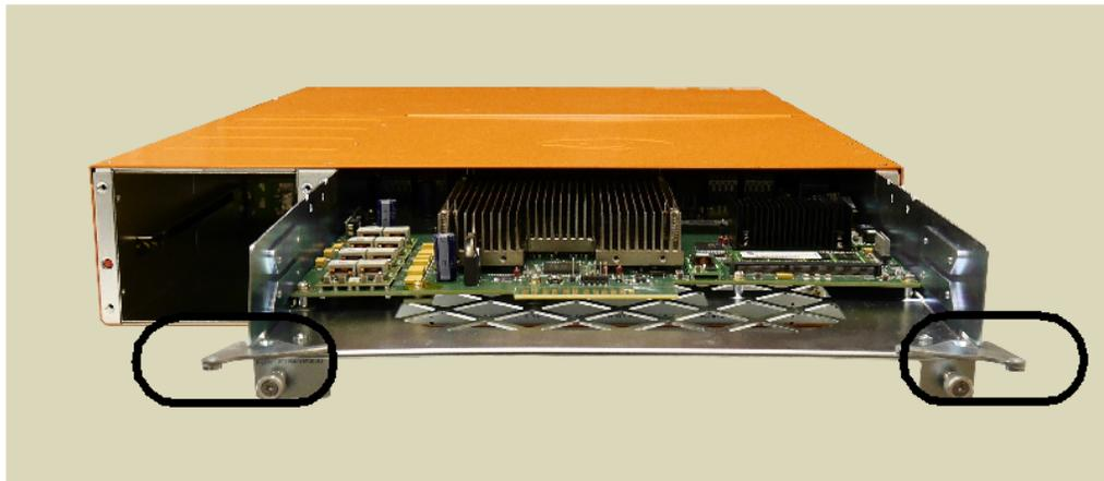
When fully inserted, close the latches on the two back corners and attach the screws into the frame.
