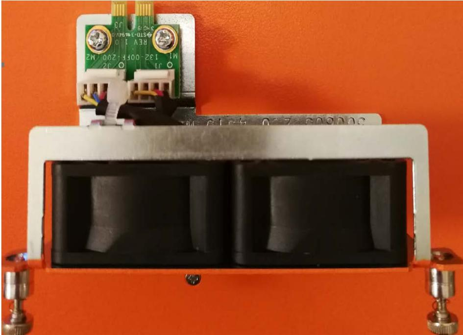
4. Insert the new fan tray in to the chassis with care.
