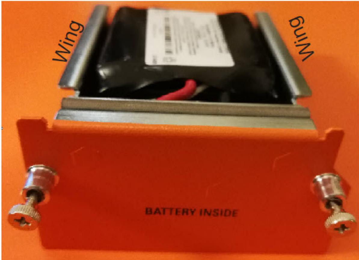
7. Orient the battery tray to insert it into the chassis
