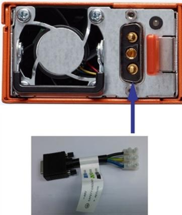
**Figure 4** Connecting DC Power Supply Module
