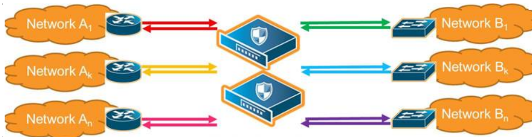
Figure 87 Inline Tool Inserted in Multiple NetA-NetB Links
