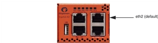
Figure 109 Stack Port Location on GigaVUE-HC1 Front
