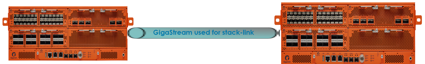
Figure 4 Daisy-Chain Configuration using GigaStream for Stack-link
