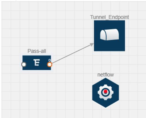
**Figure 20** Adding a link from Pass-all Map to Tunnel\_Endpoint
