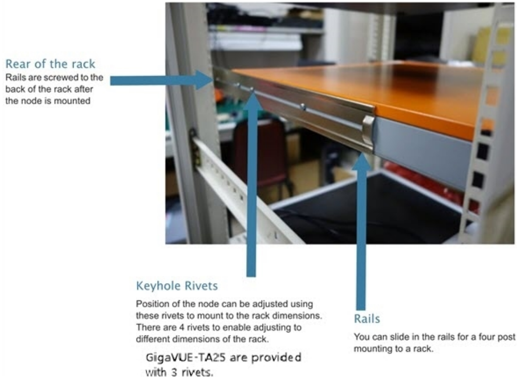
Figure 2 GigaVUE TA Series Traffic Aggregator with Rail Mounting for Four-Post Racks
