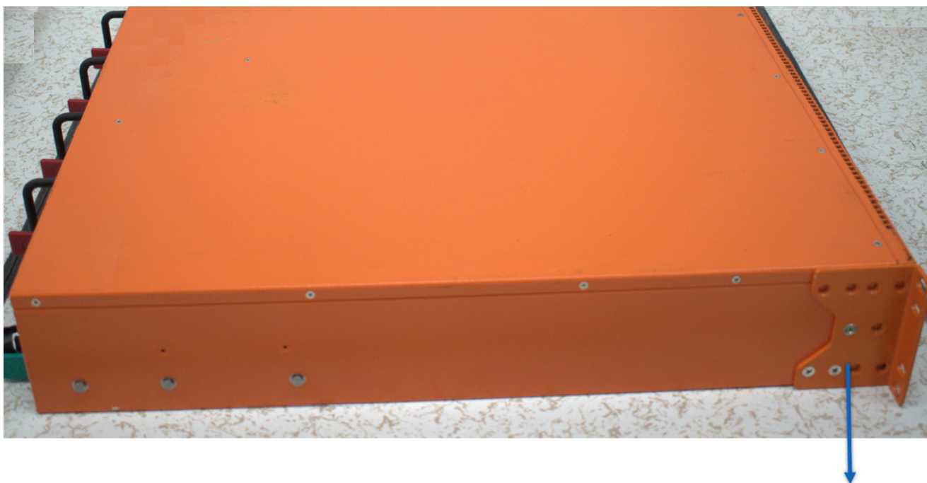
Front-Mounting Rack Ears In this picture, the rack ears are attached facing towards the front of the chassis.
