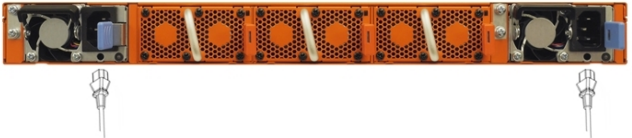
Figure 10 Connecting AC Power on a GigaVUE-TA200
