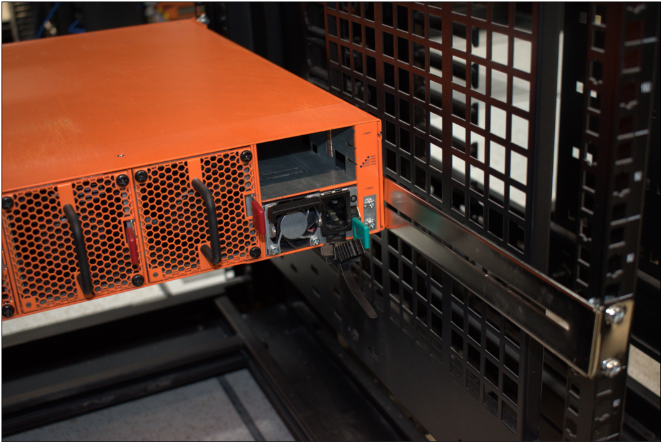
Figure 6 Rear View of the Mounted Node and Rails on the Four-Post Rack
