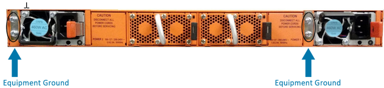
Figure 7 Ground Screws (GigaVUE TA Series Shown)
