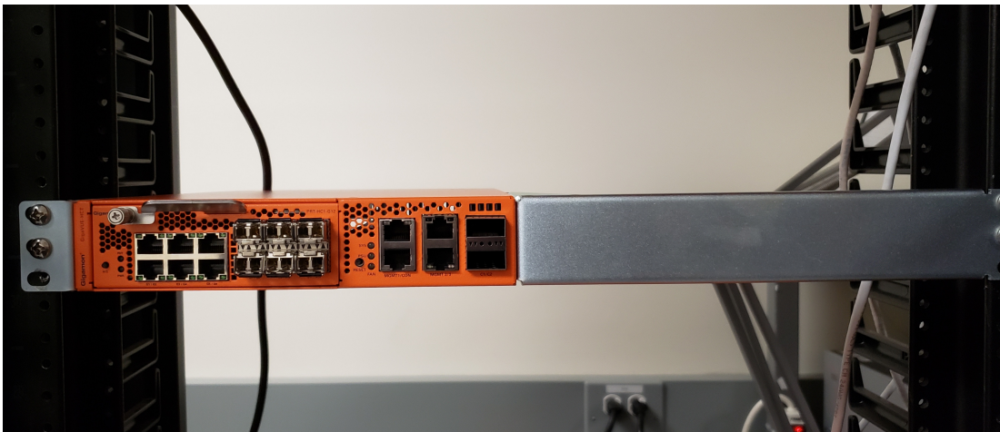
Figure 10 Four-Post Rack Installation (Single Chassis Assembly)
