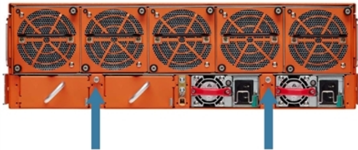
Figure 10 Fan Tray Screw Location on GigaVUE-HC3 Rear
