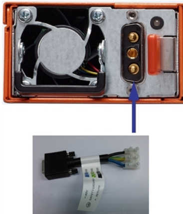
Figure 4 Connecting DC Power Supply Module
