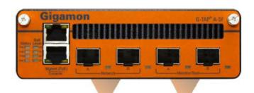
The G-TAP A-SF accepts SFP and SFP+ transceivers as well as Direct Attach Cables for the Network and Monitor/Tool ports. The transceivers in the Network A and B ports must match for successful traffic flow (for example, two SFP SR transceivers).
