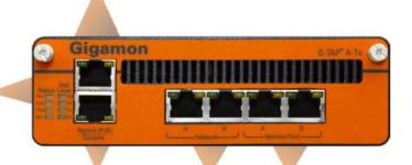
Serial Console port accepts terminal connections for configuration of G-TAP A Series settings, including time, network, and SNMP settings. Speed is configurable in CLI – default settings are 8N1, 115,200 bps.
