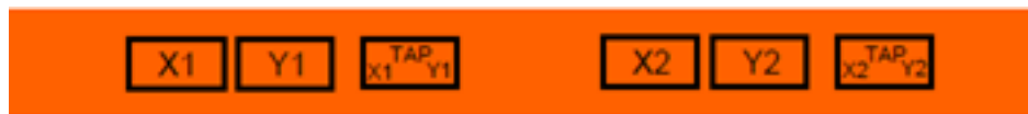
Figure 1-14: Port Label for G-TAP M251LT, M252LT, M253LT, M253ULT, M261LT, M262LT, M263LT, M271LT, M272LT, M273LT, and M273ULT
