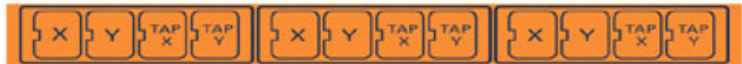
Figure 1-13: Port Label for G-TAP M451, M451T, M453T, M471, M471T, M471-SR10, and M473T
