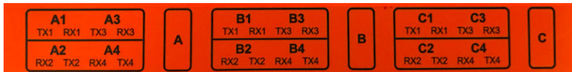
Figure 1-18: Port Label for Breakout Panels PNL-M341, PNL-M341T, PNL-M343, and PNL-M343T
