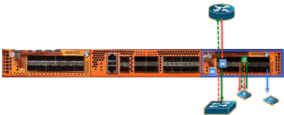
Figure 52 Logical Bypass Without Bypass Combo Module
