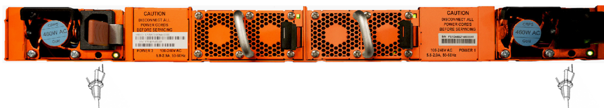
Figure 6 Connecting AC Power
