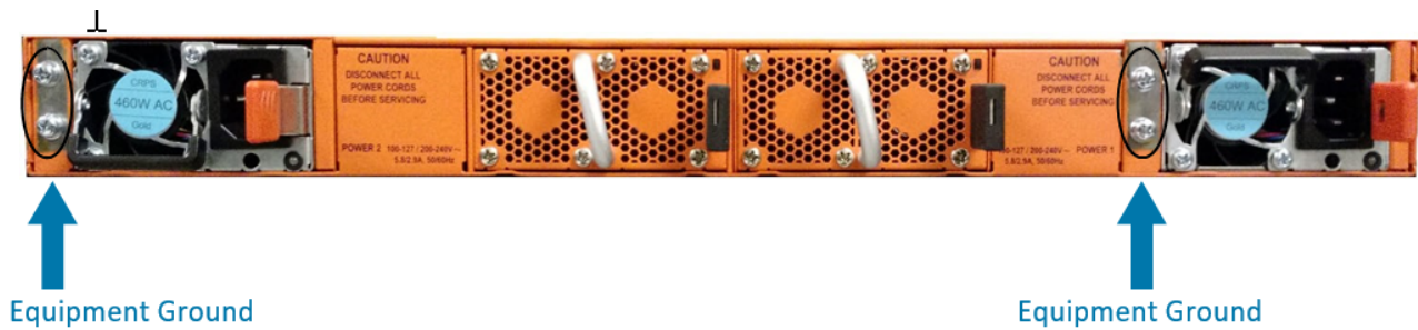
Figure 5 Ground Screws (GigaVUE-TA400E Shown)
