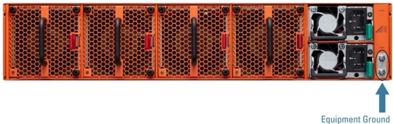
Figure 8 Ground Screws (GigaVUE TA Series-Shown)
