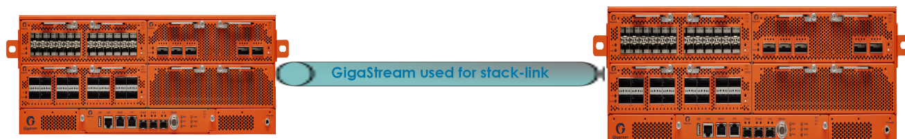
Figure 4 Daisy-Chain Configuration using GigaStream for Stack-link
