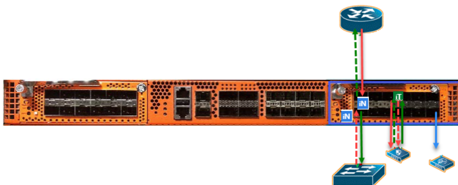
Figure 63 Logical Bypass Without Bypass Combo Module
