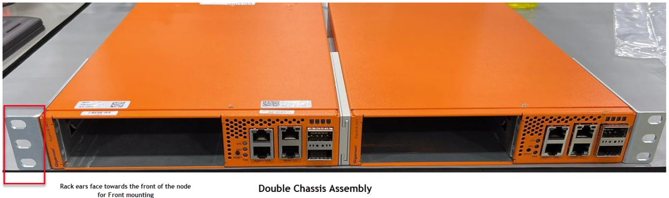
Figure 9 Rack Ears for Front Mount (Reverse Rack Ears for Center Mount)
