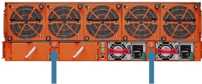
Figure 10 Fan Tray Screw Location on GigaVUE-HC3 Rear
