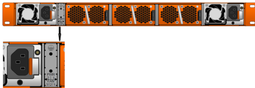
Figure 13 Holes for Ground Screws
